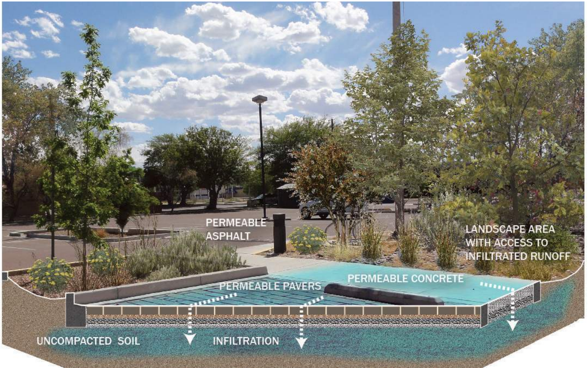
System with multiple permeable pavement types
